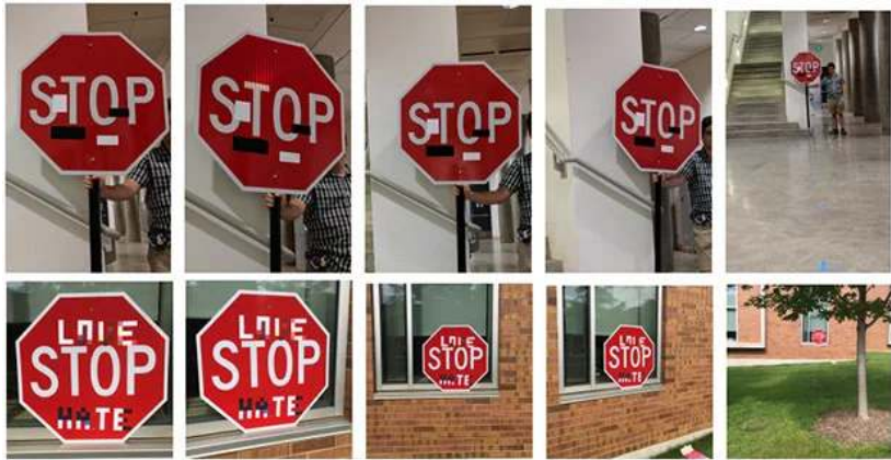
Figure 15.4: Adversarial Stickers: Nearly imperceptible stickers can trick machine learning models into misclassifying stop signs as speed limit signs over 85% of the time. This emphasizes the vulnerability of ML systems to adversarial attacks. Source: Eykholt et al. (2017).
