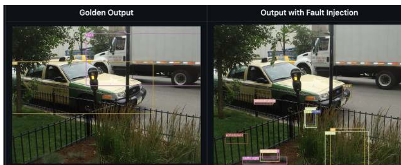
Figure 16.41: Fault Injection Effects: Bit-level hardware faults can induce phantom objects and misclassifications in machine learning models, potentially leading to safety-critical errors in applications like autonomous driving; the left image represents correct classification, while the right image presents a false positive detection resulting from a single bit flip injected using pytorchfi .
