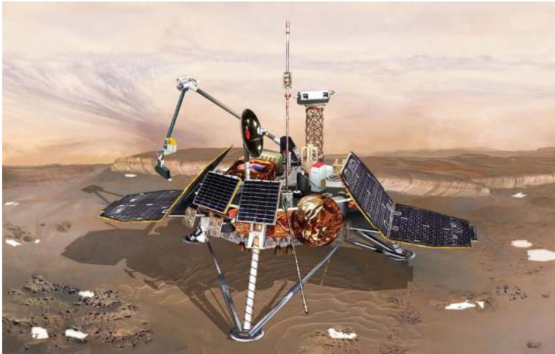
Figure 16.4: Touchdown Detection Failure: Erroneous Sensor Readings During the Mars Polar Lander Mission Triggered a Premature Engine Shutdown, Demonstrating the Critical Need for Robust Failure Modes and Rigorous Validation of Embedded Systems, particularly Those Operating in Inaccessible Environments. This Incident Underscores How Software Errors Can Lead to Catastrophic Consequences in Safety-Critical Applications and Emphasizes the Growing Importance of Reliable AI Integration in Complex Systems. Source: Slashgear.
